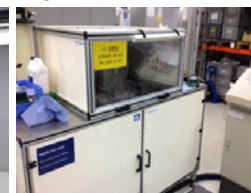
Impulse pressure test stand up to 4000 bar.
